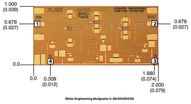
Units: millimeters (inches) Bond pad dimensions are shown to center of bond pad. Thickness: 0.110 +/- 0.010 (0.0043 +/- 0.0004), Backside is ground, Bond Pad/Backside Metallization: Gold All Bond Pads are 0.100 x 0.100 (0.004 x 0.004). Bond pad centers are approximately 0.109 (0.004) from the edge of the chip. Dicing tolerance: +/- 0.005 (+/- 0.0002). Approximate weight: 1.239 mg.
